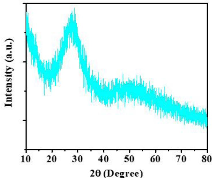
**Figure 2:** Eu<sup>3+</sup> ions concentration (mol%) dependent XRD patterns of TLLE 2.0 glass sample
