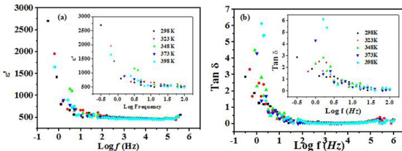
Figure 9: The frequency dependence curves at room temperature of dielectric constant  $\epsilon'(\omega)$  (a) and loss factor (b) for TLLE1.5 glass sample. Inset shows the variation of  $\epsilon'(\omega)$  and  $\tan(\delta)$  at different temperatures case of 1.5 mol%  $\text{Eu}_2\text{O}_3$
