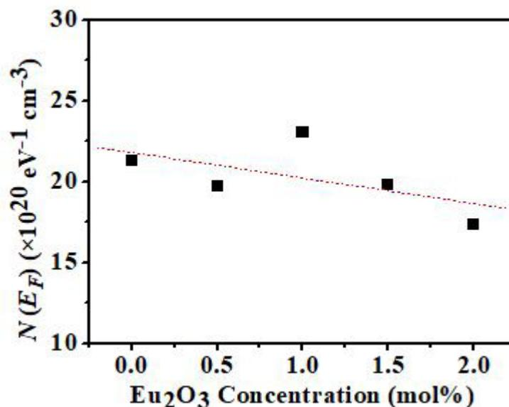
Figure 8: The calculated density of localized state,  $N(E_F)$  as function of  $\text{Eu}_2\text{O}_3$  concentration at 298 K
