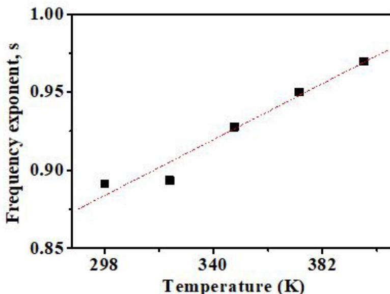
**Figure 7:** Variation of the exponent parameter,  $s$  with temperature for TLLE 2.0 glass
