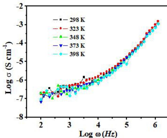
**Figure 6:** Frequency dependence of the conductivity,  $\sigma_{ac}(T)$ , at temperatures shown for the TLLE glass doped 1.5 mol% Eu<sub>2</sub>O<sub>3</sub>
