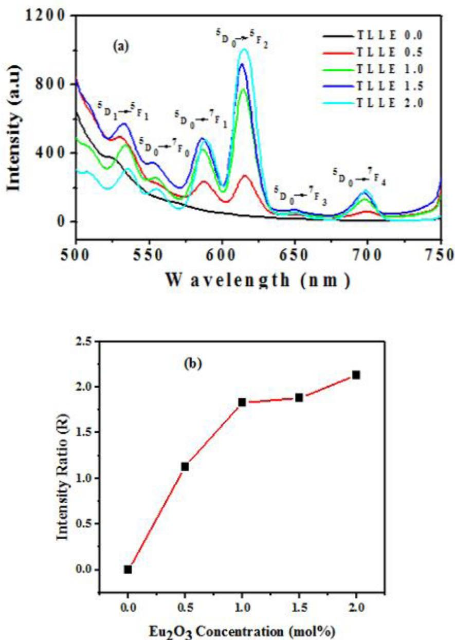
Figure 12(a): Photoluminescence spectra of the prepared glasses and (b) intensity ratio against  $\text{Eu}_2\text{O}_3$  concentration
