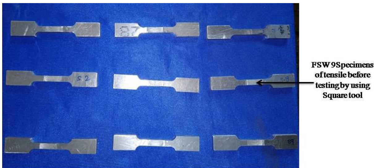
Figure 3: Specimens of Tensile test before testing with ASTM E8
