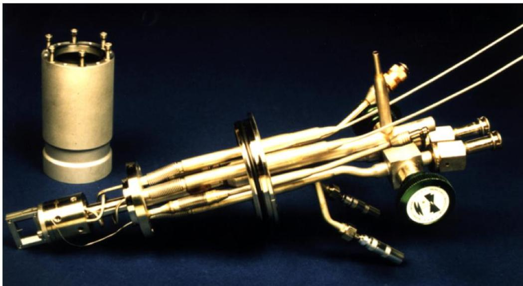
**Figure S2:** Details of the *in-situ* cell in use for the *Guinier* system. The separately shown cylindrical cup made of Beryllium defines the volume ( $\approx 115$  ml) of the reaction cell. It will be attached to the lower water-cooled flange. Note the circular groove, etched down to a thickness of 0.3 mm to allow for the transmission of the X-ray beam.
