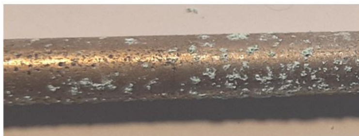
Figure 6: Damages on the surface of Ni-anode (5.4 mm in diameter) after one hour of operation in the water electrolysis mode.
